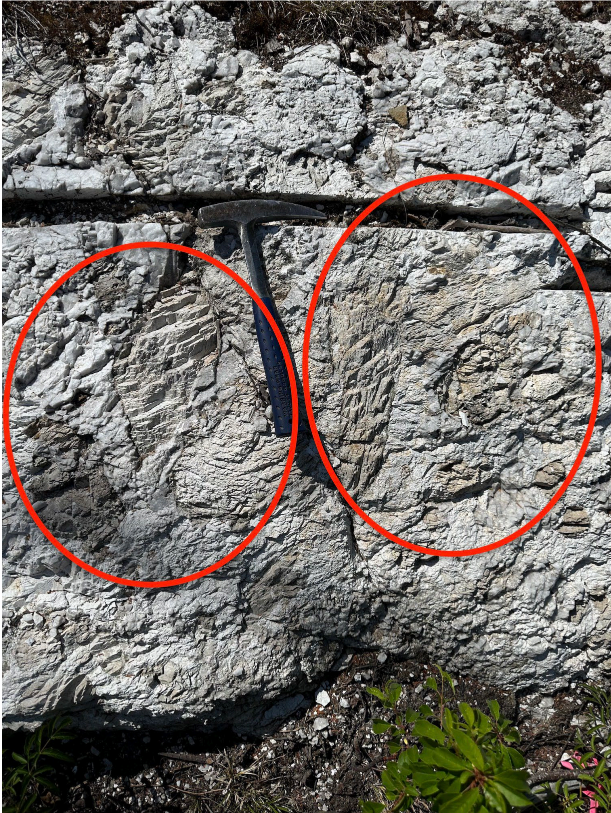
FIGURE 7.7 SPODUMENE IN JACKPOT PEGMATITE DYKE
