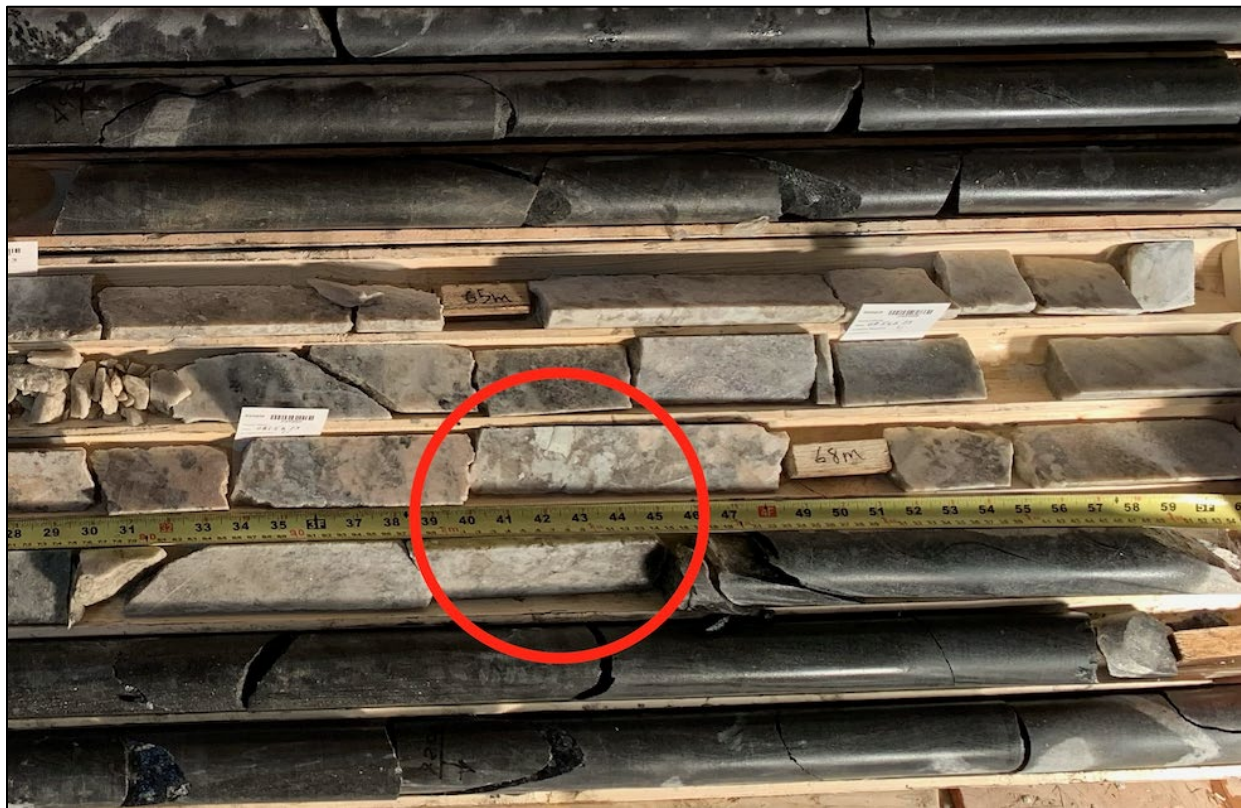
FIGURE 7.8 SPODUMENE IN DRILL HOLE JP-2023-04
